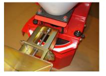
**3.** Insert the (removed) feed block into the Calibration Hopper, ensure the drive shaft aligns by slowly rotating the feed shaft
