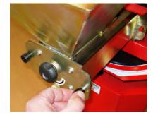
5. Place a suitable container under the Calibration Hopper to collect pellets whilst calibrating
