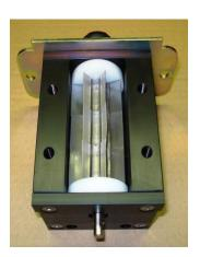
When re-fitting the end plates to the feed block after changing the configuration, the end plate should be able to fit flush with the feed block by hand, without having to pull it home with the socket head screws.
