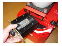
**2.** Slide the Calibration Hopper into the Fan Jet in place of the feed block with the hopper uppermost, ensure the drive shaft aligns and secure with the supplied screw knobs.
