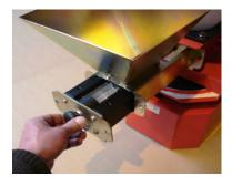
**4.** Secure with the two small blacks PVC knobs supplied.
