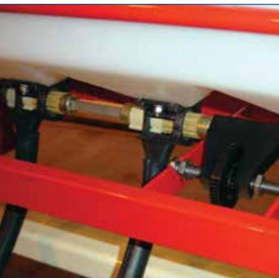
**The application rate is set** by a combination of feed aperture setting and shaft speed - which in turn is a combination of gearbox setting (high or low speed) and feed motor speed. For 2 or 3 metre units, each hopper has its own adjuster to slide the 6 feed rolls together.
